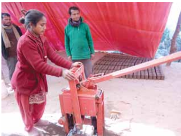
Compressed stabilized earthen brick (CSEB) being produced by Dalit community (Thokarpa, Sindupalchowk) The brick was used to construct 120 houses in Thokarpa.
